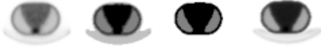
Fig. 1. Illustration of the segmentation process of the heart/chest phantom transmission images showing from left to right: the original transmission image, FCM segmented image using 5 clusters, merging process to a three-clustered image, and the final attenuation map after applying a Gaussian filter and weighted averaging.
