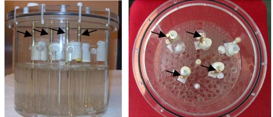
Figure 1. Photo of the Jaszczak phantom with 4 metallic inserts (arrows).
