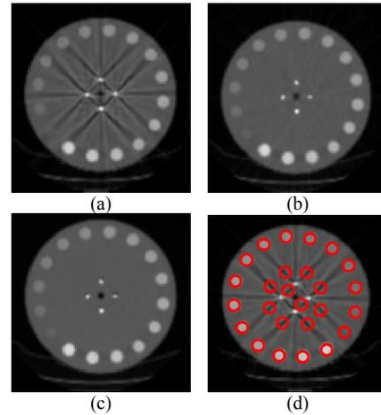
**Figure 3.**  $\mu$ map obtained from (a) the original image, (b) the corrected image, (c) metal artifact-free image. (d) ROIs defined on the  $\mu$ map to evaluate the accuracy of the metal artifact reduction technique.
