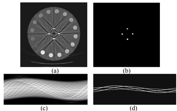
Figure 2. Detection of affected projections: (a) original CT image, (b) metal only image, (c) original sinogram and (d) metal-only sinogram.
