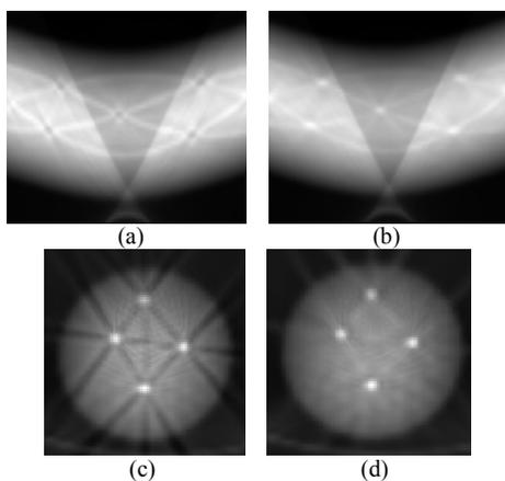
**Figure 5.** ACF sinograms generated by the PET/CT scanner using (a) non corrected CT image, (b) corrected CT image. (c)  $\mu$ map before correction, (d)  $\mu$ map obtained after MAR.
